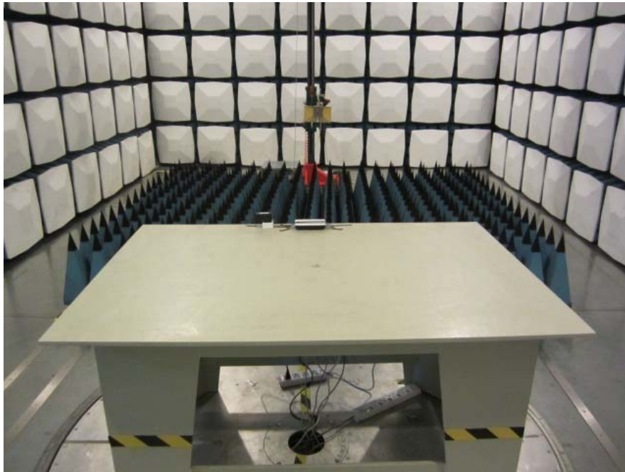
Radiated Emission -Front View (Above 1GHz)
