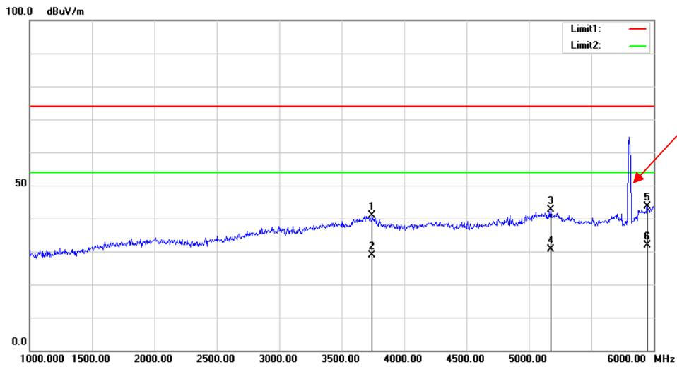
Fundamental Test with Band Rejection Filter
