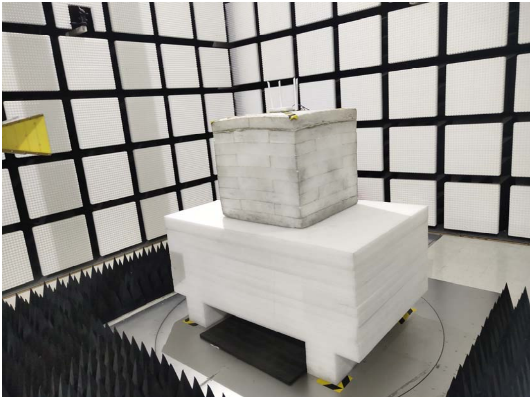
Radiated Emission Above 1GHz View
