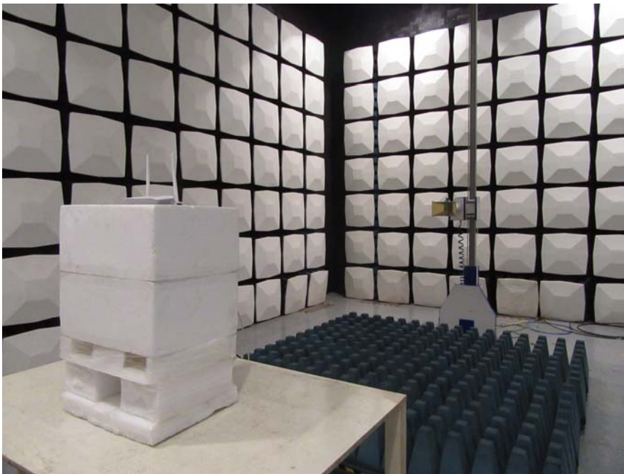
Radiated Emission View (Above 1GHz)
