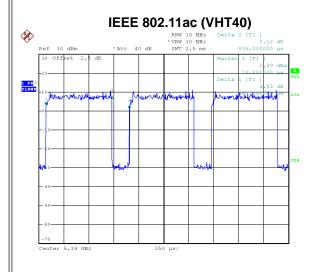
Duty cycle = 0.660 ms / 0.835 ms = 79.04%Duty Factor =  $10 * \log(1 / \text{Duty cycle}) = 1.02 \text{ dB}$
