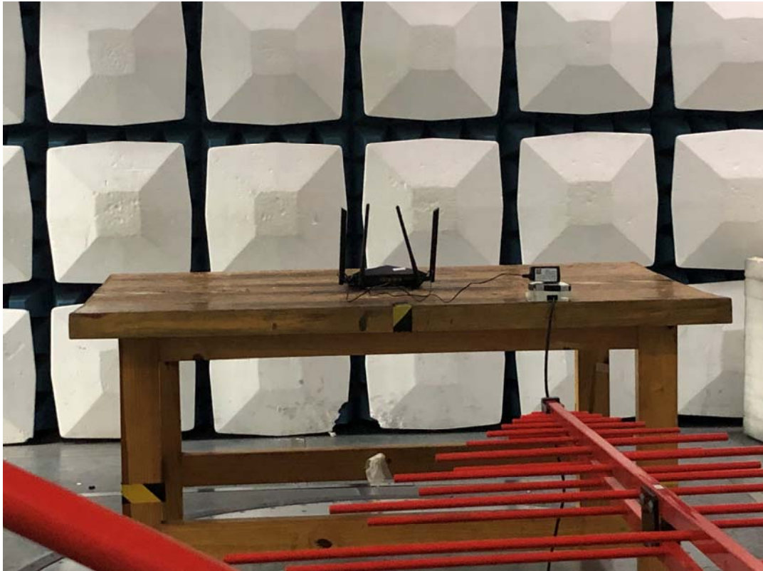
Radiated Emission Above 1GHz View
