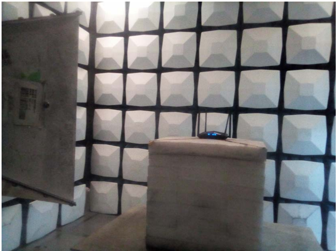
Radiated Emission Above 1GHz View
