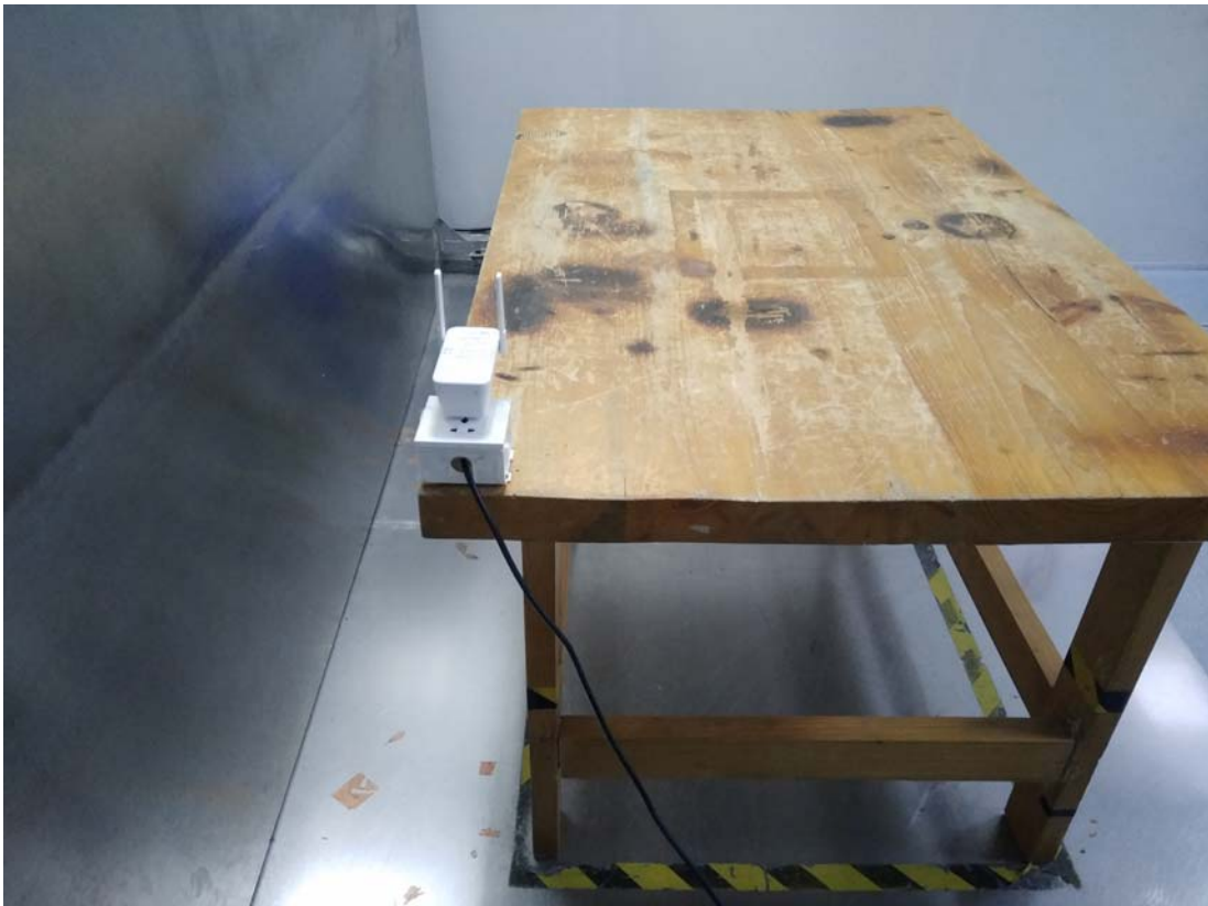
Conducted Emissions Side View
