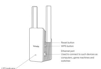
Solid blue: Extended successfully. Proper position or too close to the router Solid yellow: Extended successfully. Fair position. Move the extender closer to the router Solid red: Extended successfully. The extender is too far away from the router Blinking red slowly: Startup completes. Not extended or failed to extend Blinking red fast: Extending by WPS button
