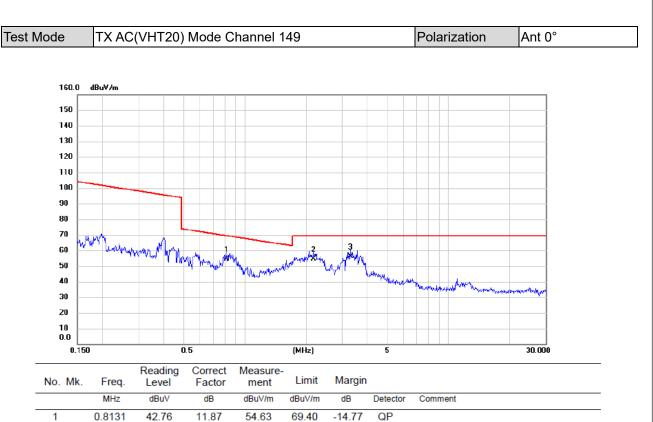
(1) Measurement Value = Reading Level + Correct Factor.
