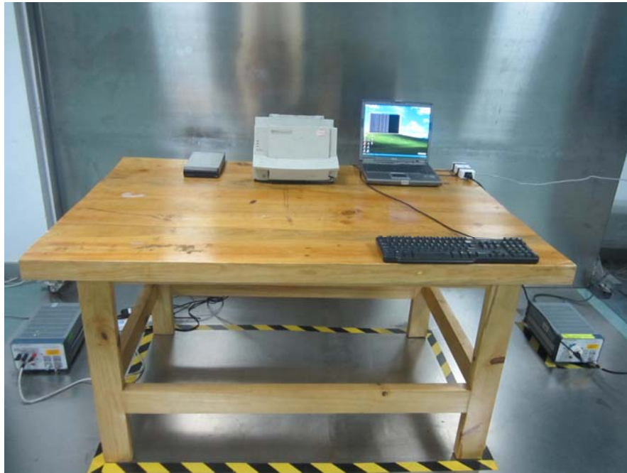
Conduction Emissions - Side View
