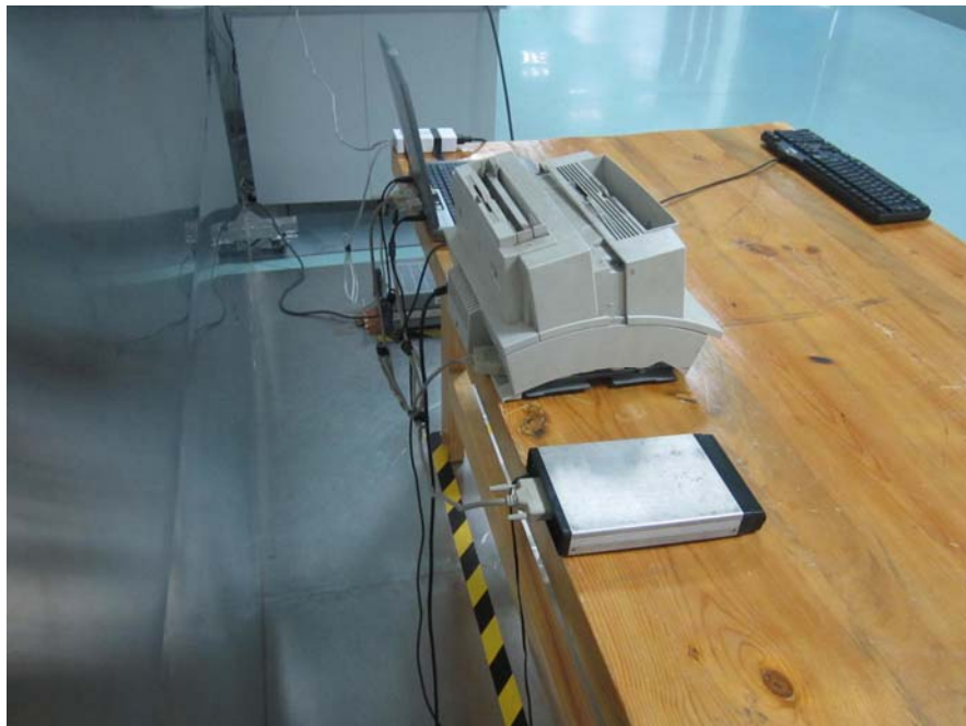
Conduction Emissions - Side View
