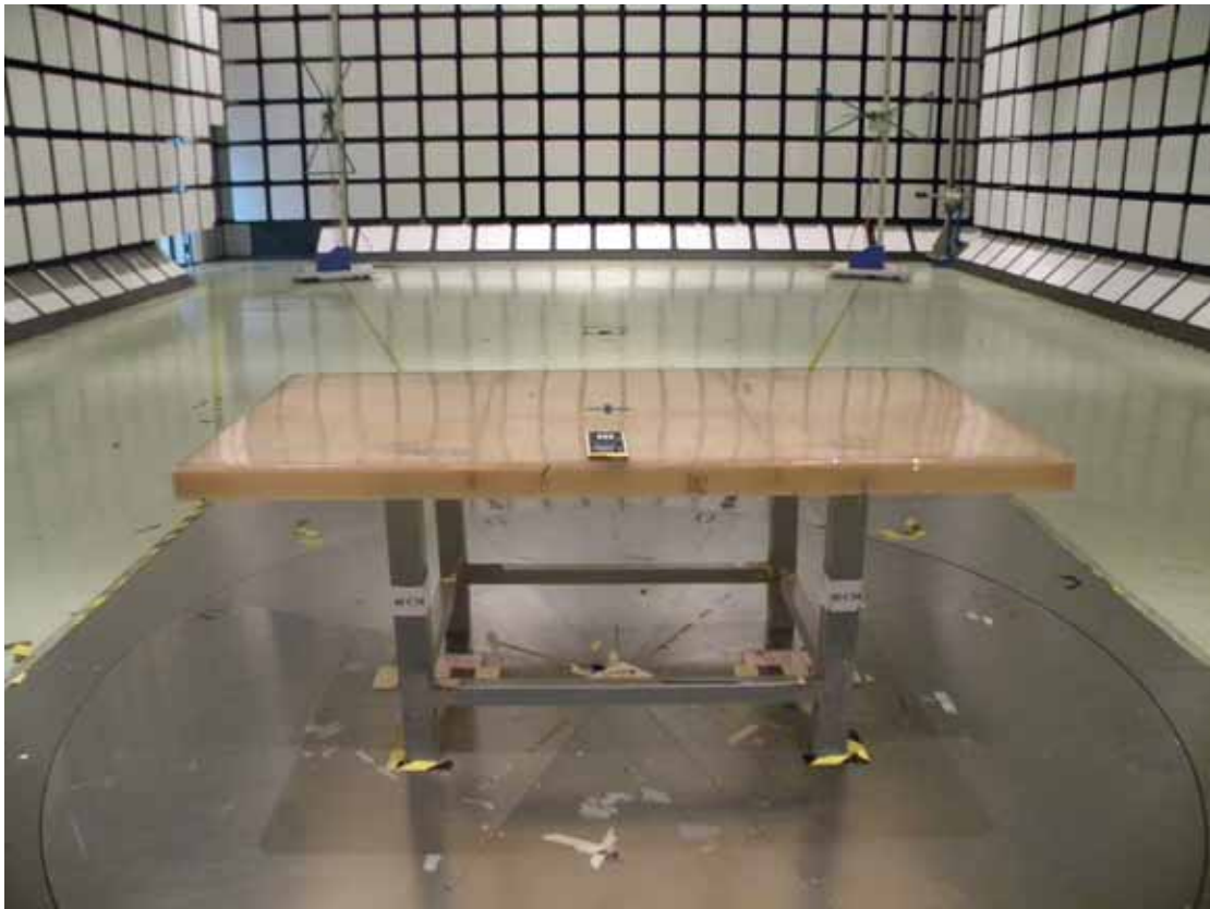
Back View of Radiated Measurement (For Configuration 1,3)
