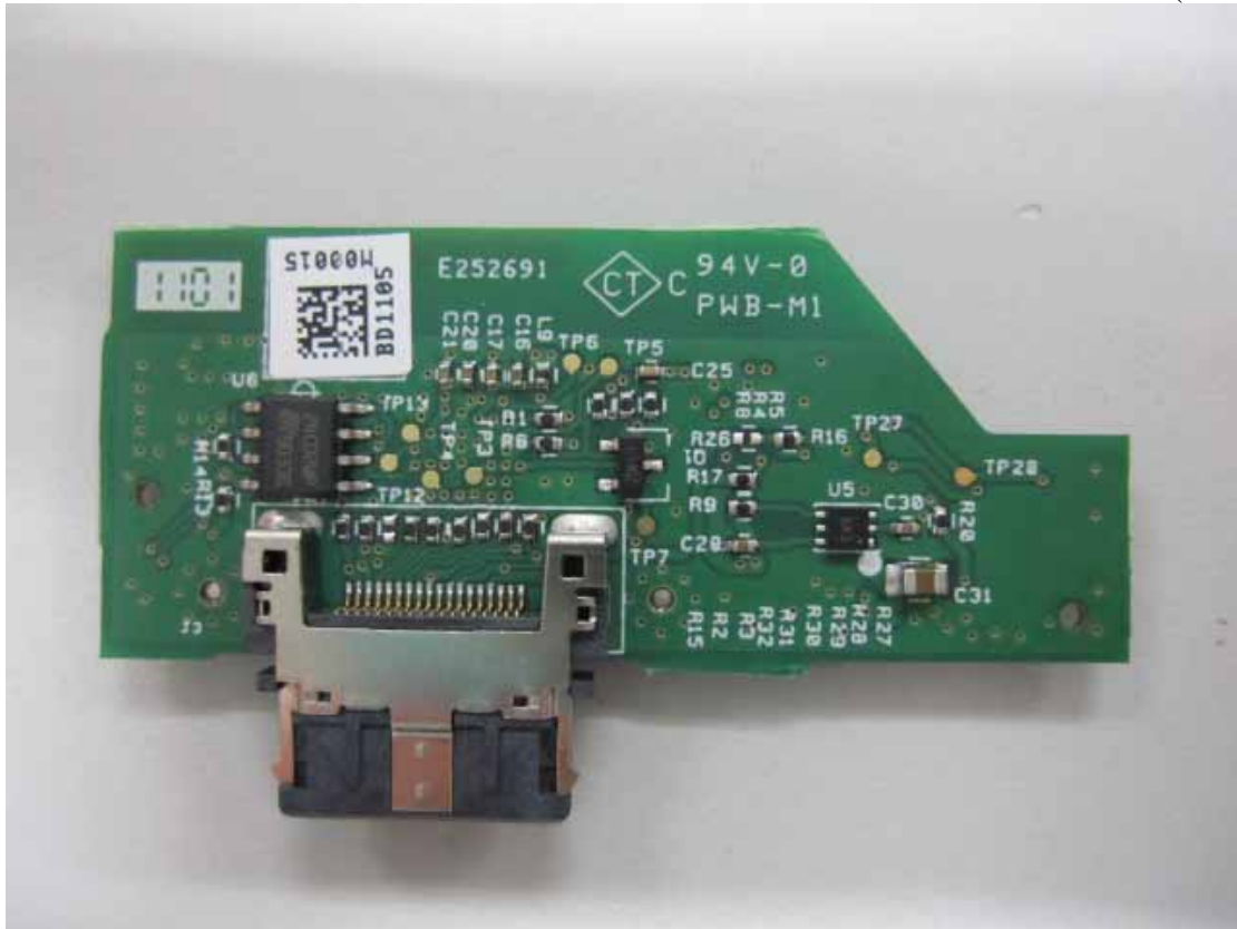
Figure 3 Wireless Module (Solder Side)
