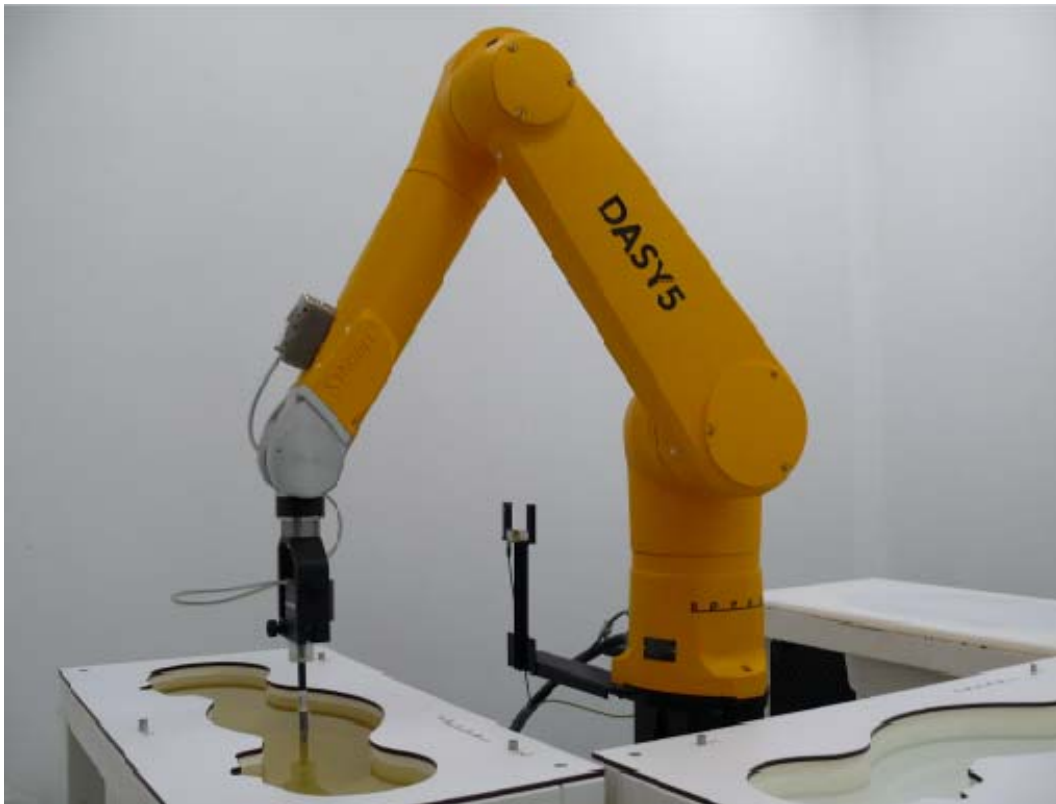
Picture 1: Specific Absorption Rate Test Layout
