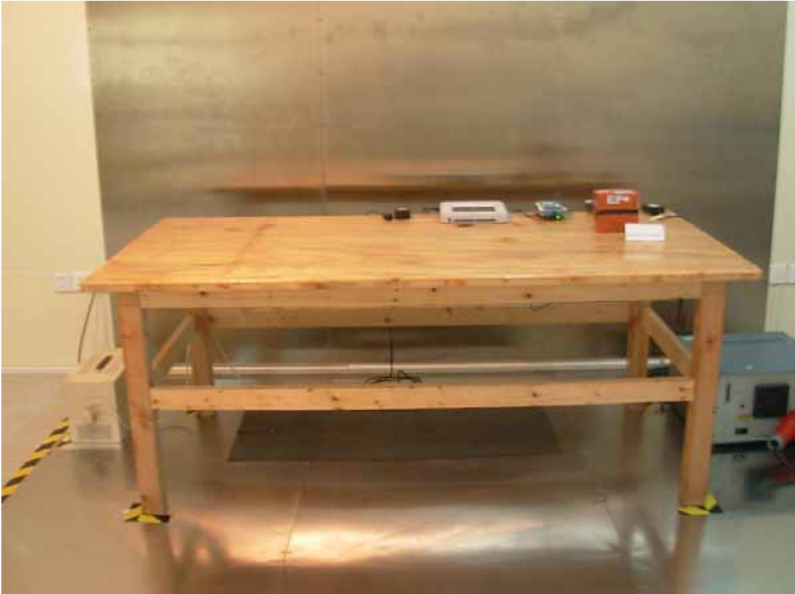
Front View of Conducted Measurement (Test Configuration A)
