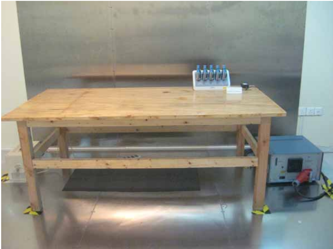
Front View of Conducted Measurement (Test Configuration C)
