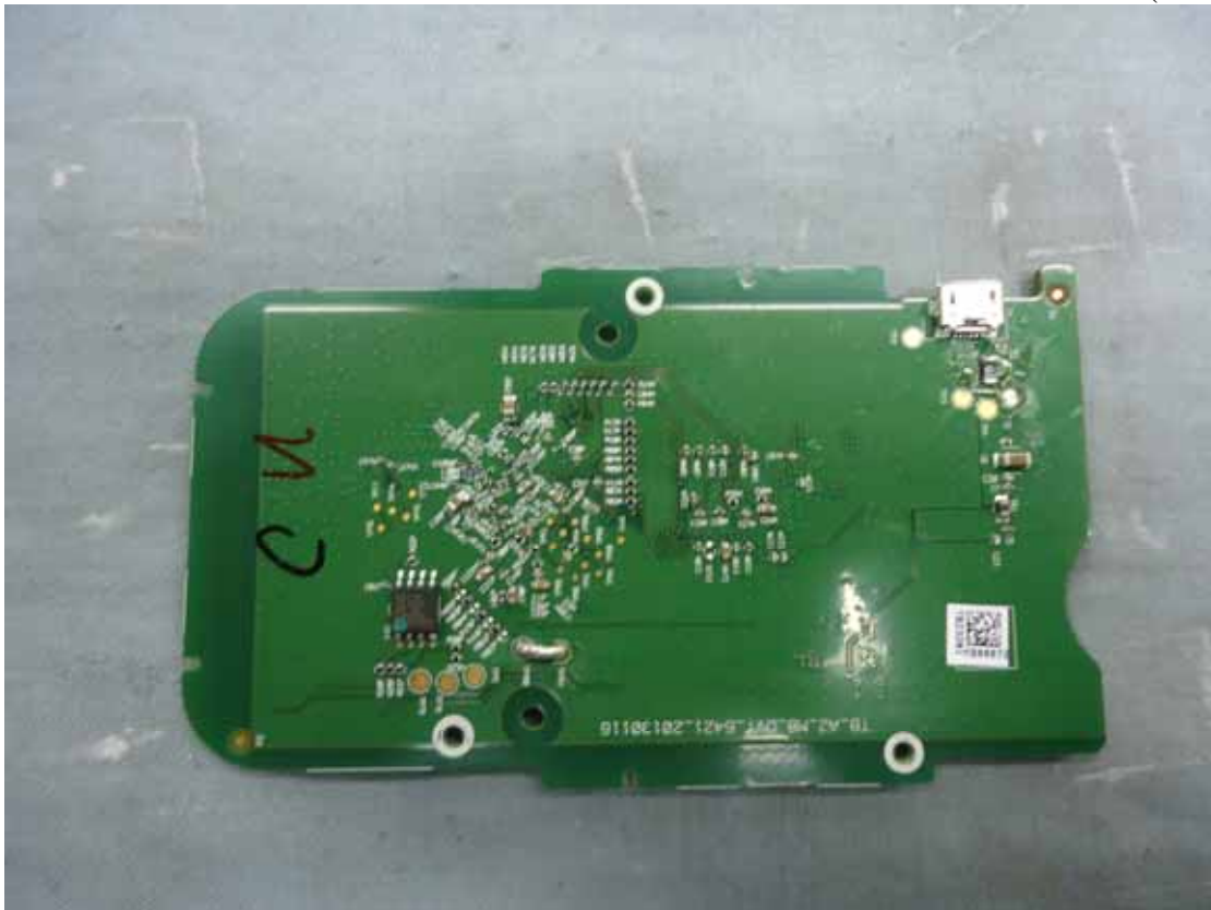
Figure 6 Wireless Module (Solder Side)
