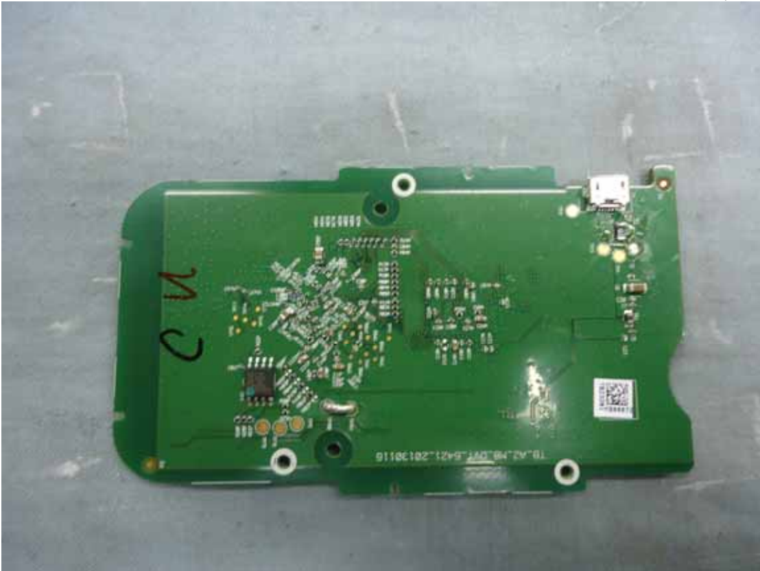
Figure 6 Wireless Module (Solder Side)
