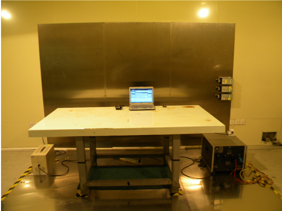
Front View of conducted emission measurement
