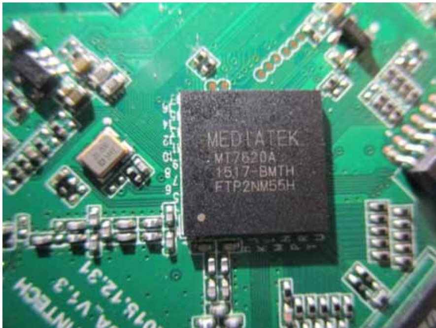
EUT –RF Chip View
