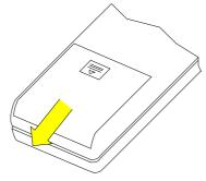
Attach the Battery to the connector inside. Put the Battery into the compartment.
