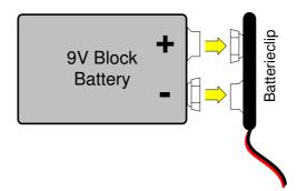
Slide the door back to close it. Use only 9V E-Block alkaline Batteries of the Type 6LR61.
