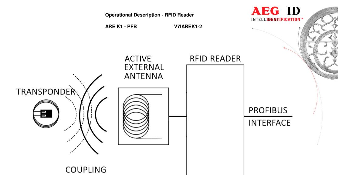
For reading a passive transponder, the RFID reader is generating an electromagnetic field. This happens when the reader is receiving a command. The electromagnetic field is powering the transponder which is modulating its UID on the exitation field. The reader receives the signal, demodulates the UID and transfers it via Profibus.
