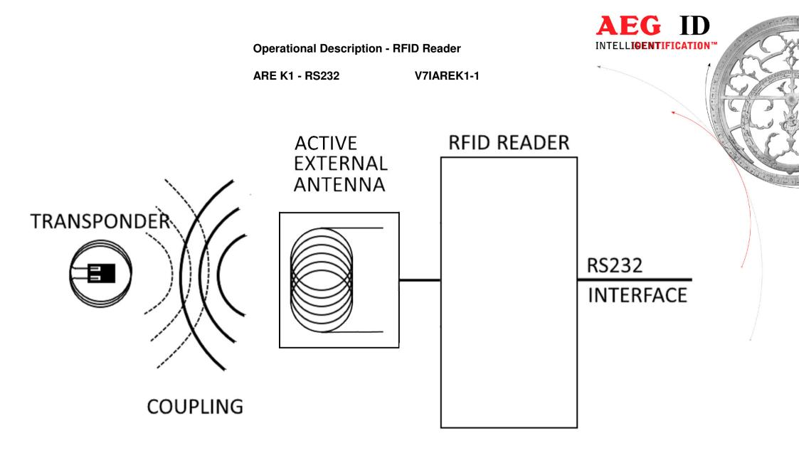
For reading a passive transponder, the RFID reader is generating an electromagnetic field. This happens, depending on the operation mode, permanently or when the reader is receiving a command. The electromagnetic field is powering the transponder which is modulating its UID on the exitation field. The reader receives the signal, demodulates the UID and transfers it via RS232.
