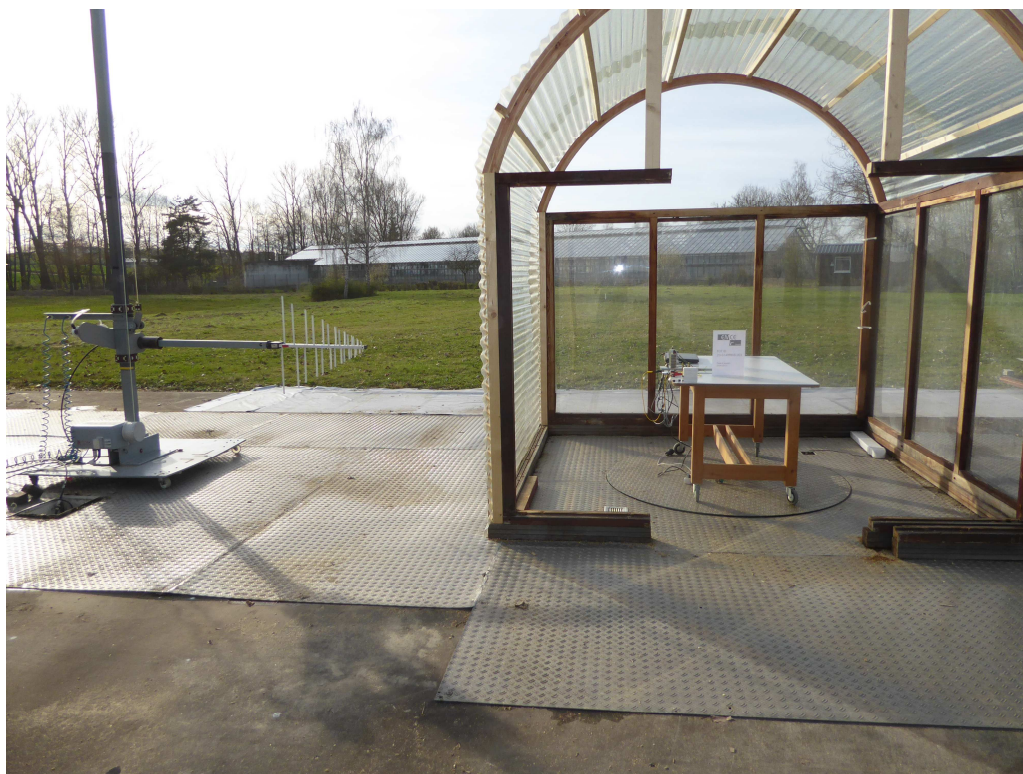
Precompliance test setup
