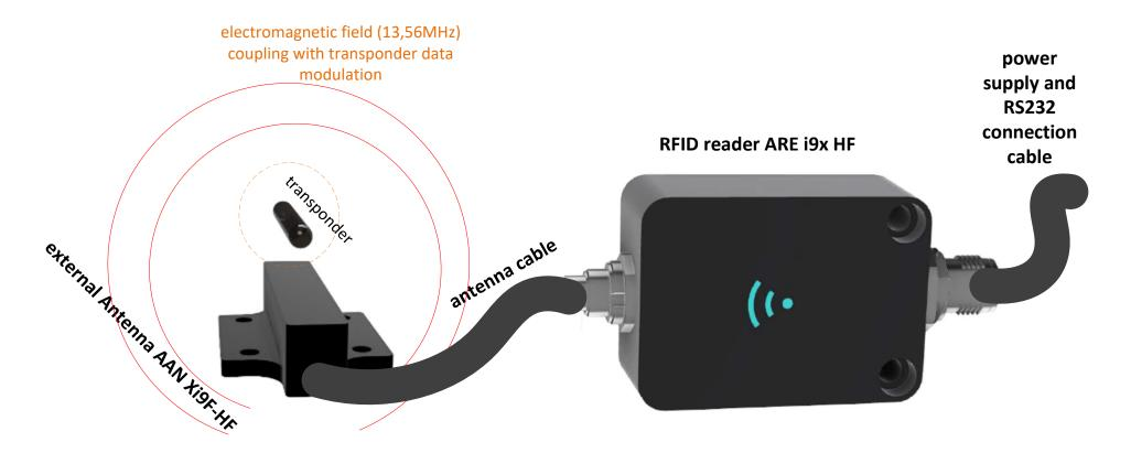
The passive transponder is powered by the energy of electromagnetic field generated by the external reader antenna, powered by the RFID reader. This happens, when the reader receives a command to the read transponder data and the transponder ist within the interrogation zone (coupling area of the electromagnetic field).
