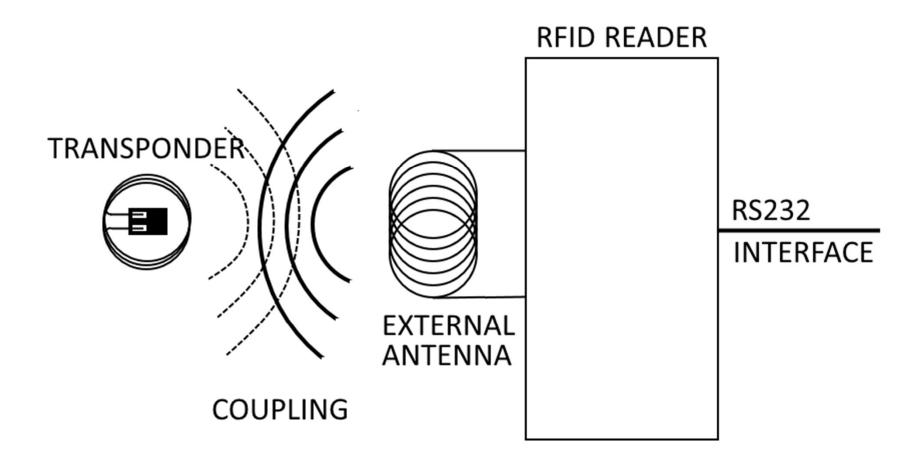
For reading a passive transponder, the RFID reader is generating an electromagnetic field. This happens, depending on the operation mode, permanently or when the reader is receiving a command. The electromagnetic field is powering the transponder which is modulating its UID on the exitation field. The reader receives the signal, demodulates the UID and transfers it via RS232.
