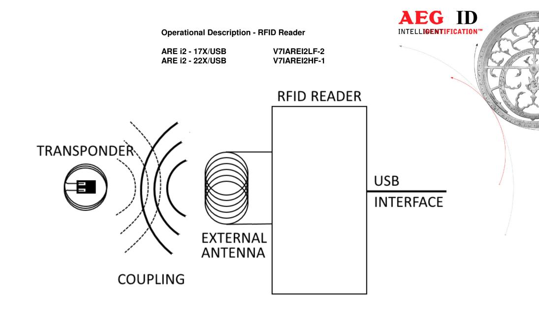
For reading a passive transponder, the RFID reader is generating an electromagnetic field. This happens, depending on the operation mode, permanently or when the reader is receiving a command. The electromagnetic field is powering the transponder which is modulating its UID on the exitation field. The reader receives the signal, demodulates the UID and transfers it via USB.
