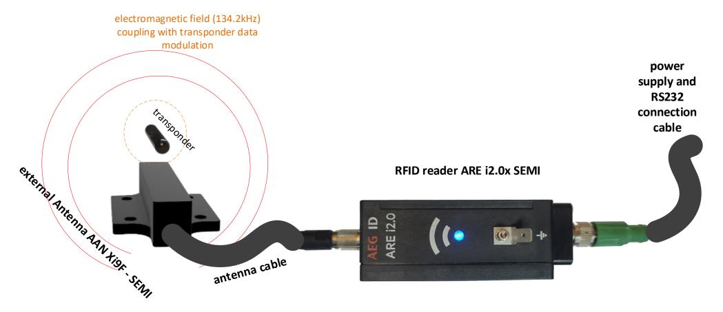
The passive transponder are powered by the energy of electromagnetic field generated by the external reader antenna, powered by the RFID reader. This happens, when the reader receives a command to the read transponder data and the transponder ist within the interrogation zone (coupling area of the electromagnetic field).
