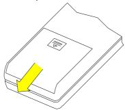
Attach the rechargeable batteries (ID-no. 1005048) as shown on the label inside the battery compartment.
