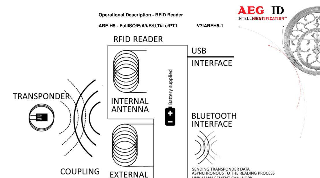
For reading a passive transponder, the RFID reader is generating an electromagnetic field. Only with one antenna. This happens triggered manualy by pressing a reader button. The electromagnetic field is powering the transponder which is modulating its UID on the exitation field. The reader receives the signal, demodulates the UID and transfers it via USB or Bluetooth.
