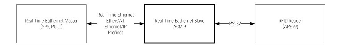
The ACM 9 (AEG ID Communication Module) is working as an interface adpater an real time Ethernet (EtherCAT, Ethernet/IP and Profinet) and RS232. It is communicating with up to 4 AEG ID RFID readers (ARE i9 LF, ARE i9 HF) and does transfer this communication to a real time Ethernet. That way the real time Ethernet Master in the network has access on the RFID readers using the ACM9.
