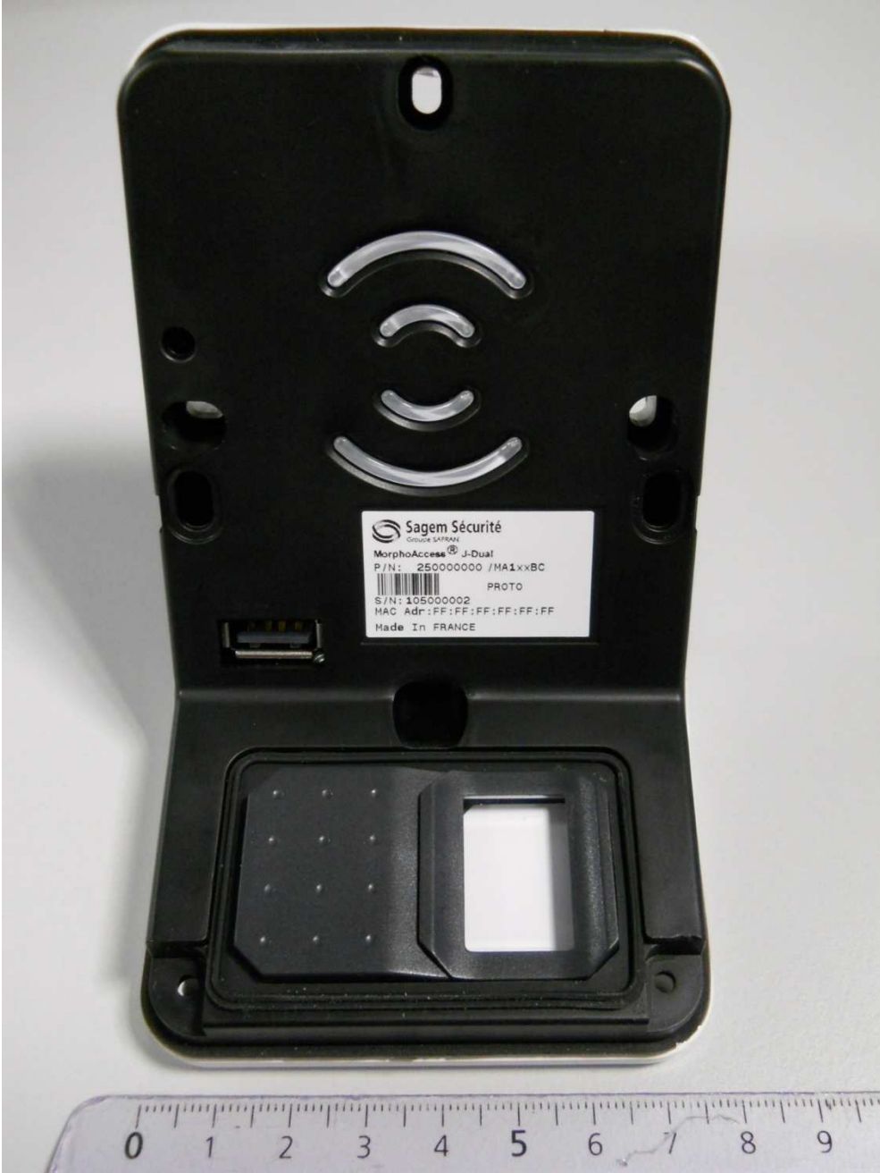
ExtPho-1 : Front side of product without front cover (smoked glass)
