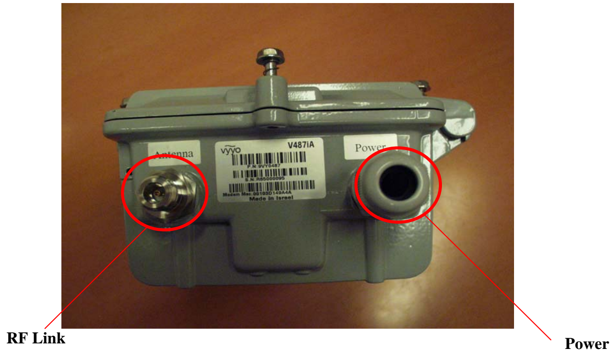
Figure 2-2: V487i WMU Rear Panel Connectors
