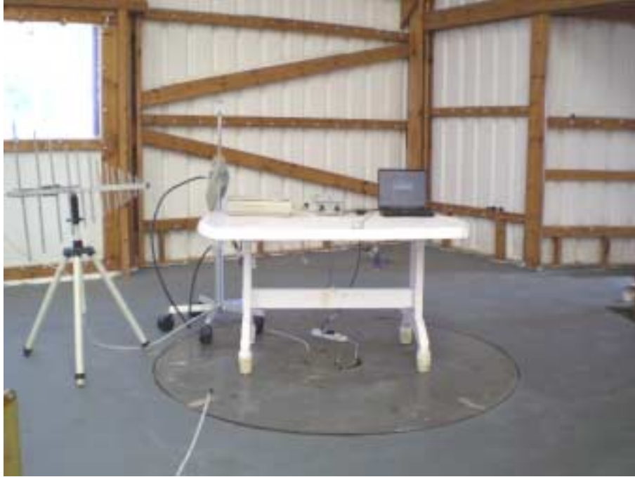
Photograph No.7 Setup for spurious emission field strength measurements at the OATS
