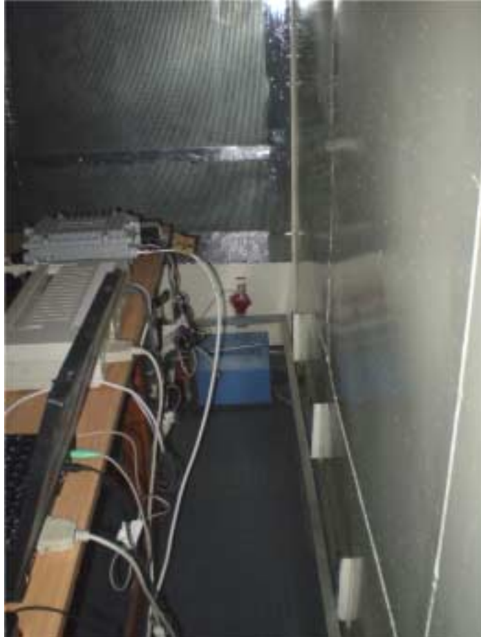
Photograph No.11 Setup for conducted emission measurements at the mains power port
