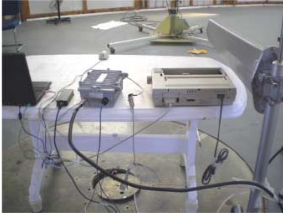
Photograph No.8 Setup for spurious emission field strength measurements at the OATS, close view
