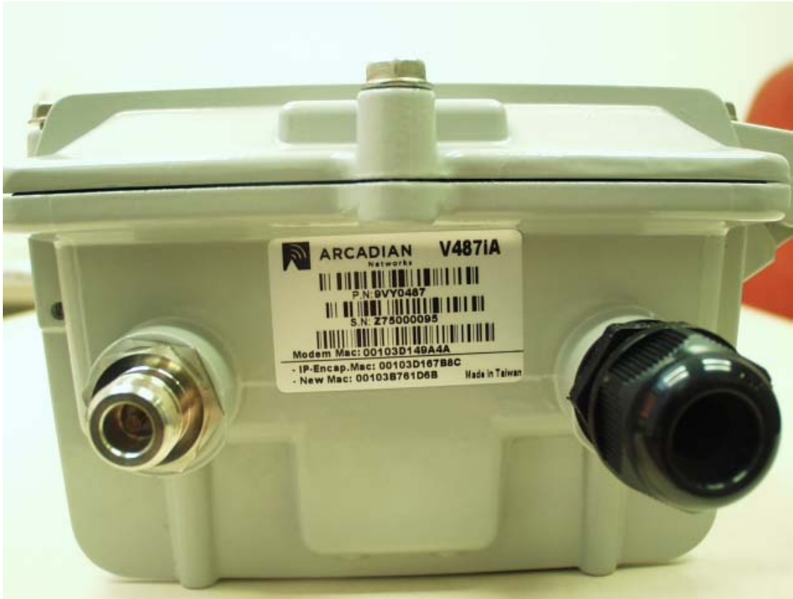
Picture 3: V487 external box connectors - RF and Power, and label
