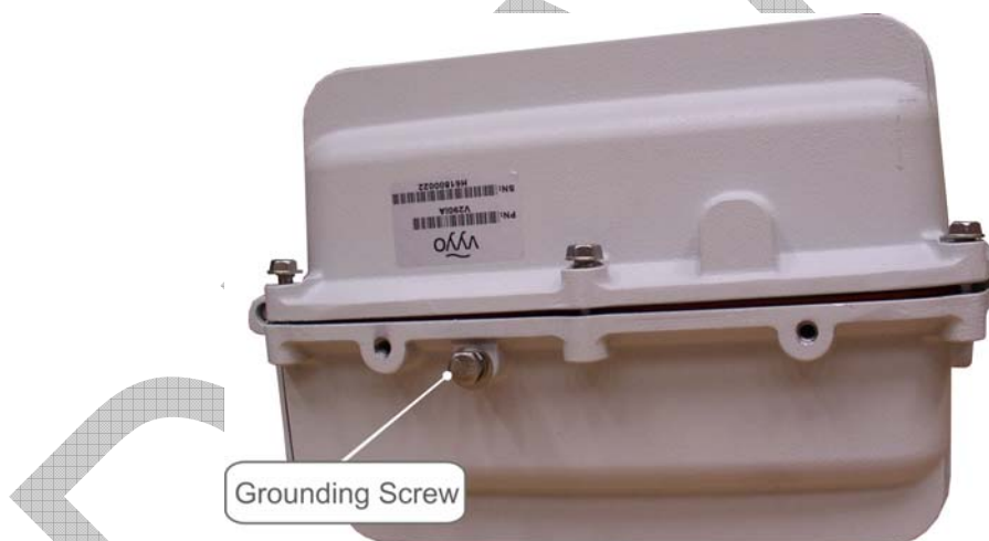
Figure 7: Attaching to Ground
