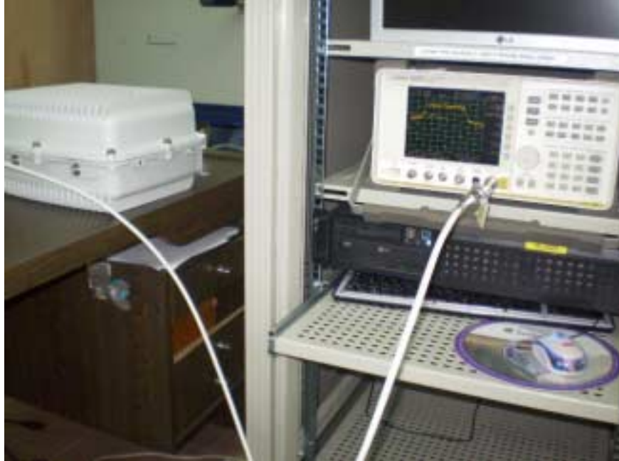
Photograph No.1 Peak output power, occupied bandwidth and spurious emissions at RF antenna connector test setups
