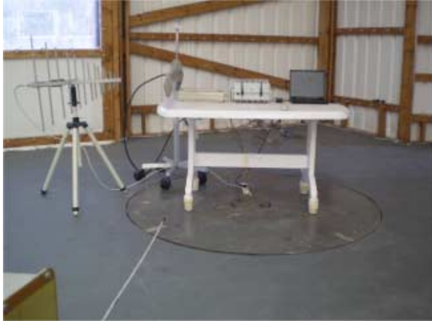
Photograph No.6 Setup for spurious emission field strength measurements at the OATS
