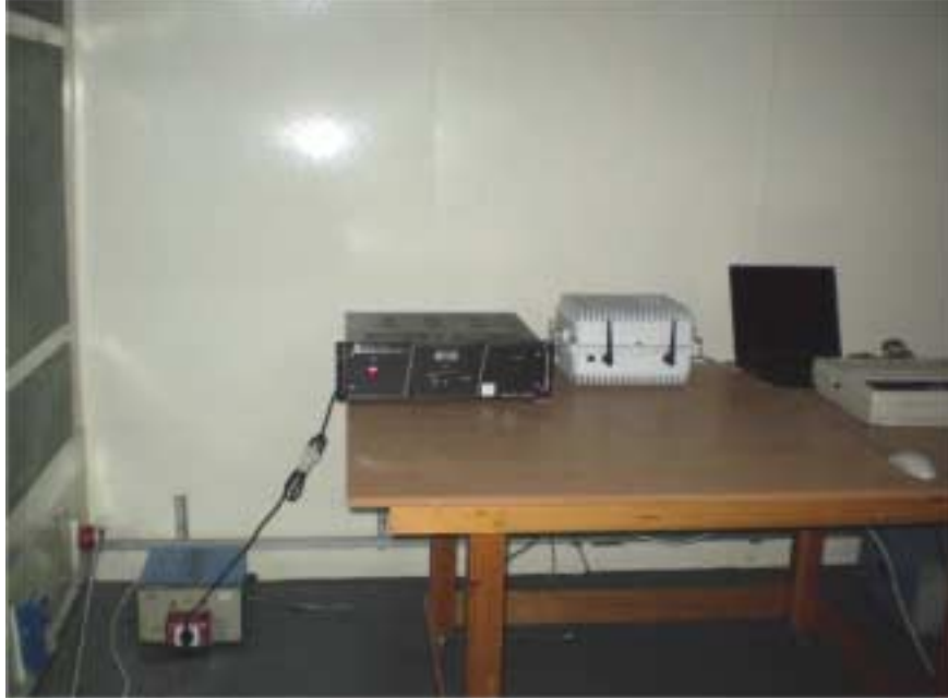
Photograph No.7 Setup for conducted emission measurements at the mains power port
