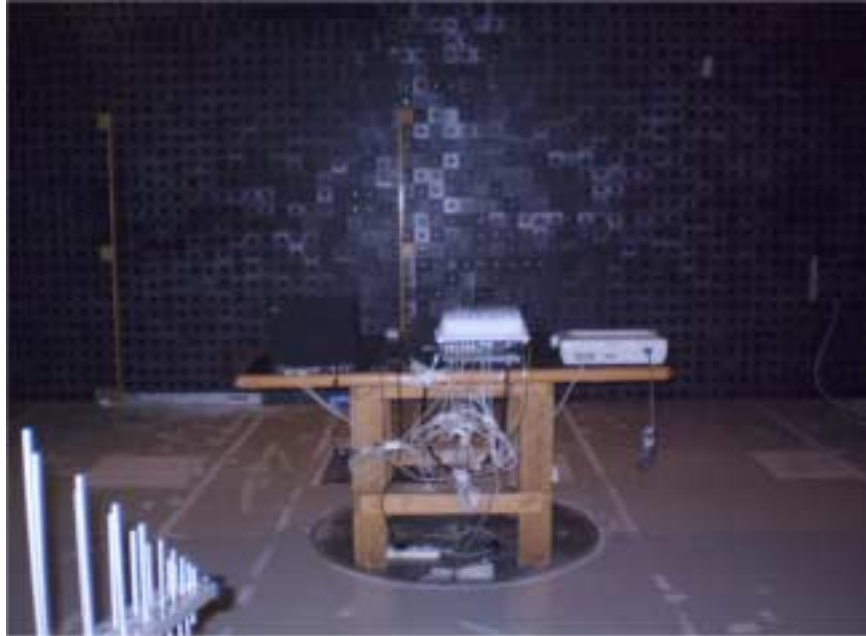
Photograph No.3 Setup for spurious emission field strength measurements in 30 MHz to 1 GHz range in the anechoic chamber
