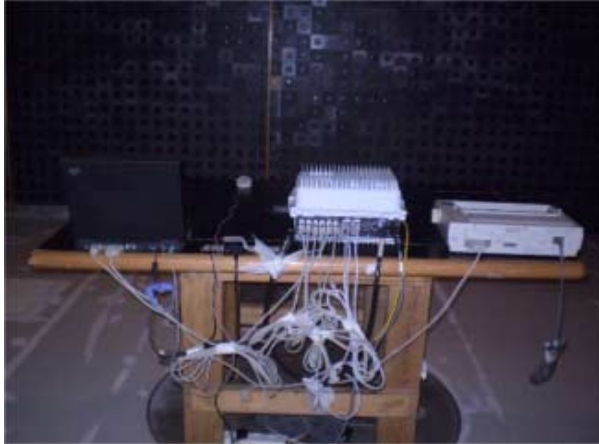
Photograph No.5 Setup for spurious emission field strength measurements close view
