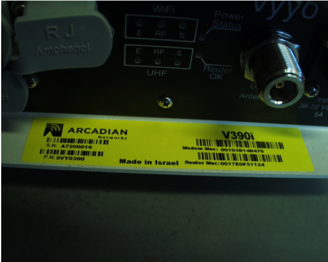
Picture 5: V390 external box connector side – RF connector and label
