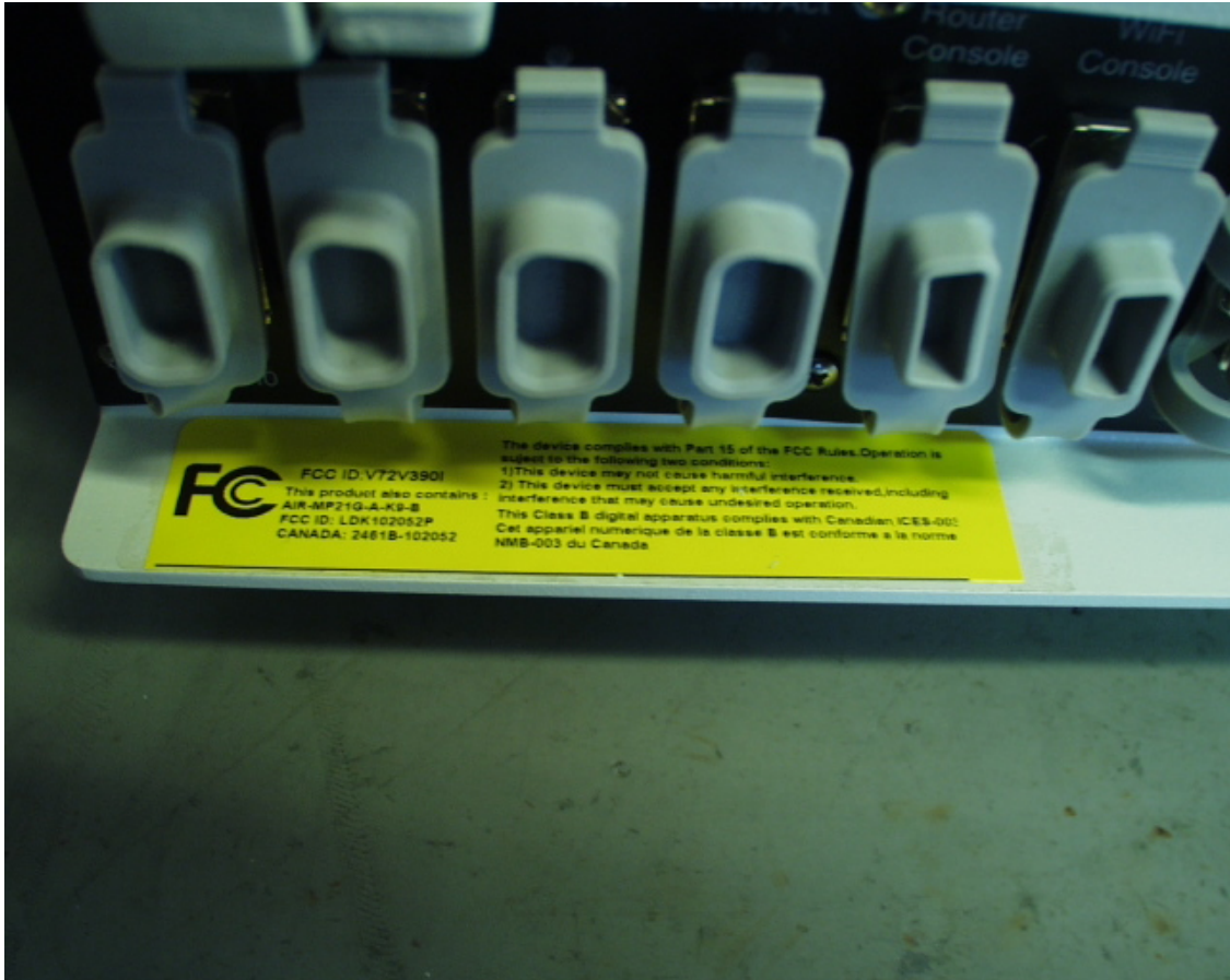
Picture 4: V390 external box connector side – LAN connectors and FCC label
