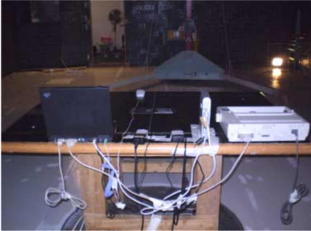
Photograph No.6 Setup for spurious emission field strength measurements close view
