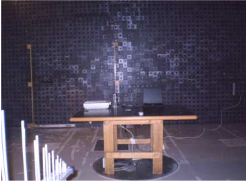
Photograph No.4 Setup for spurious emission field strength measurements in 30 MHz to 1 GHz range in the anechoic chamber
