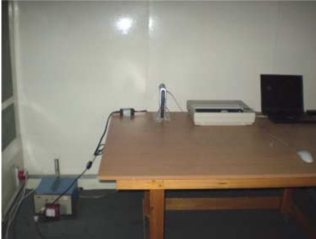
Photograph No.10 Setup for conducted emission measurements at the mains power port
