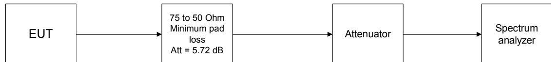
Figure 7.4.1 Occupied bandwidth test setup
