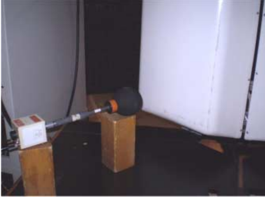
Photograph No.7 Maximum permissible exposure (MPE) measurement setup, close view
