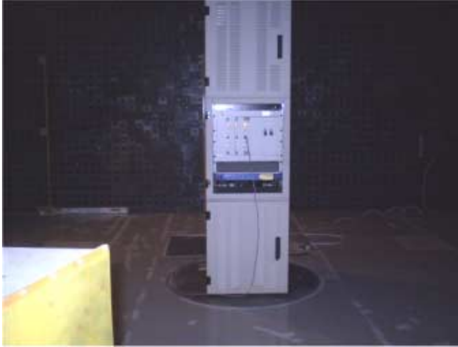
Photograph No.5 Setup for spurious emission field strength measurements above 1 GHz range in the anechoic chamber
