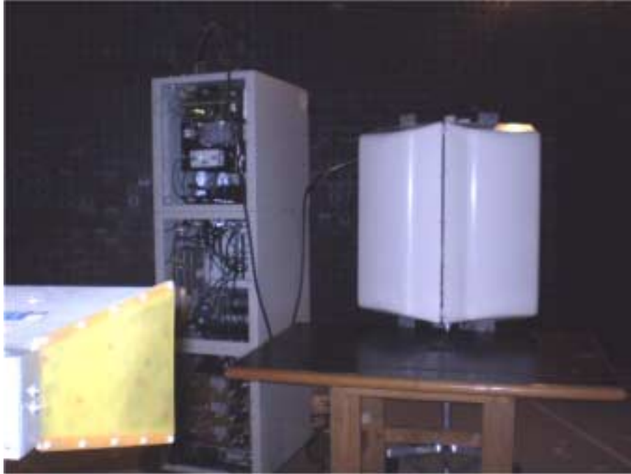
Photograph No.6 Maximum permissible exposure (MPE) measurement setup
