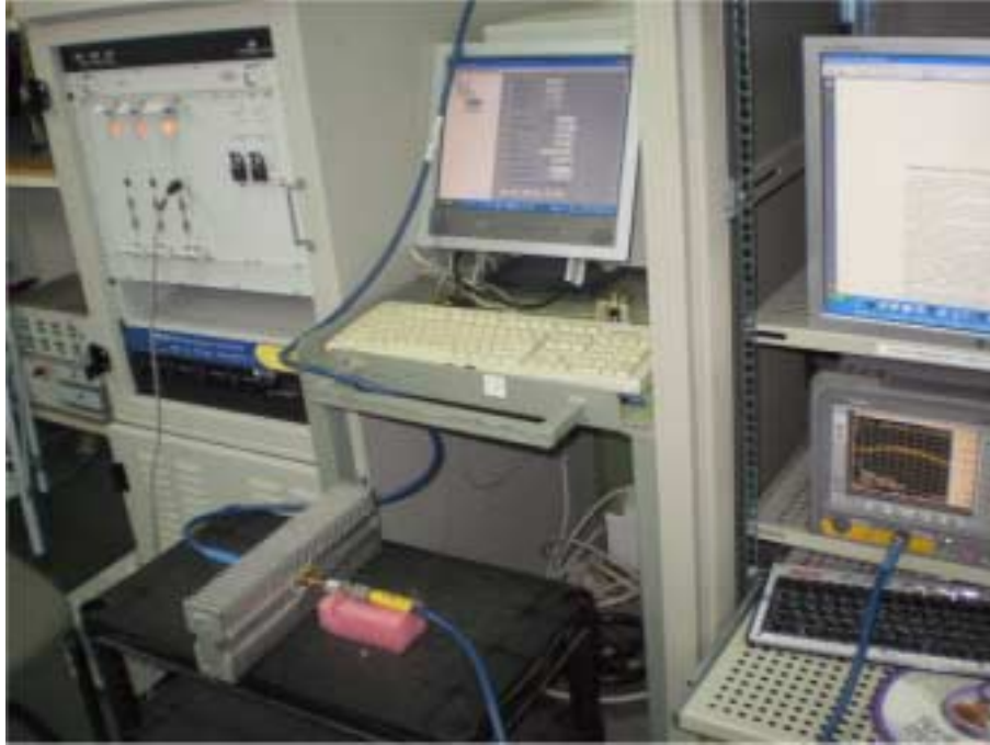
Photograph No.2 Peak output power, occupied bandwidth and spurious emissions at RF antenna connector test setups
