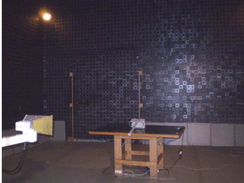
Photograph No.3 Setup for spurious emission field strength measurements above 1 GHz range in the anechoic chamber
