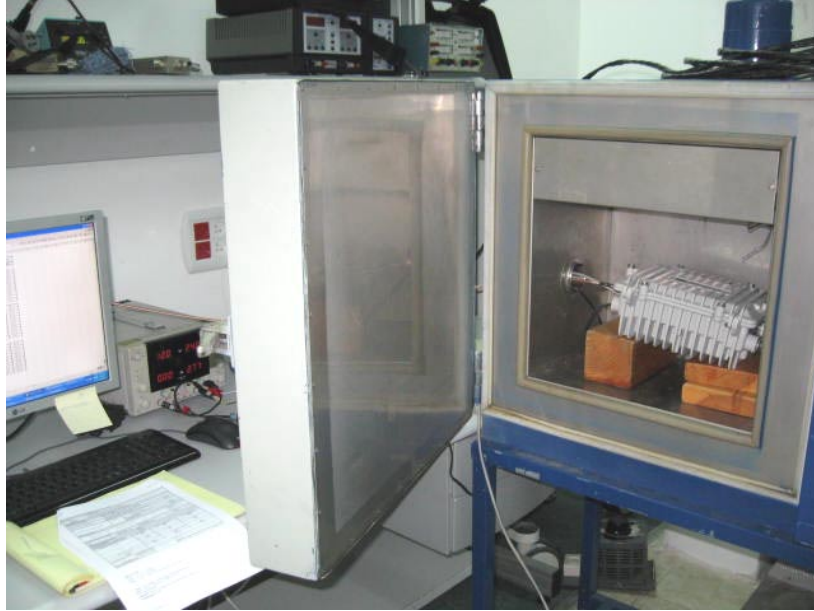
Photograph No.6 Setup for frequency stability measurements
