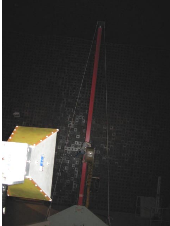
Photograph No.5 Setup for substitution method measurements in the anechoic chamber
