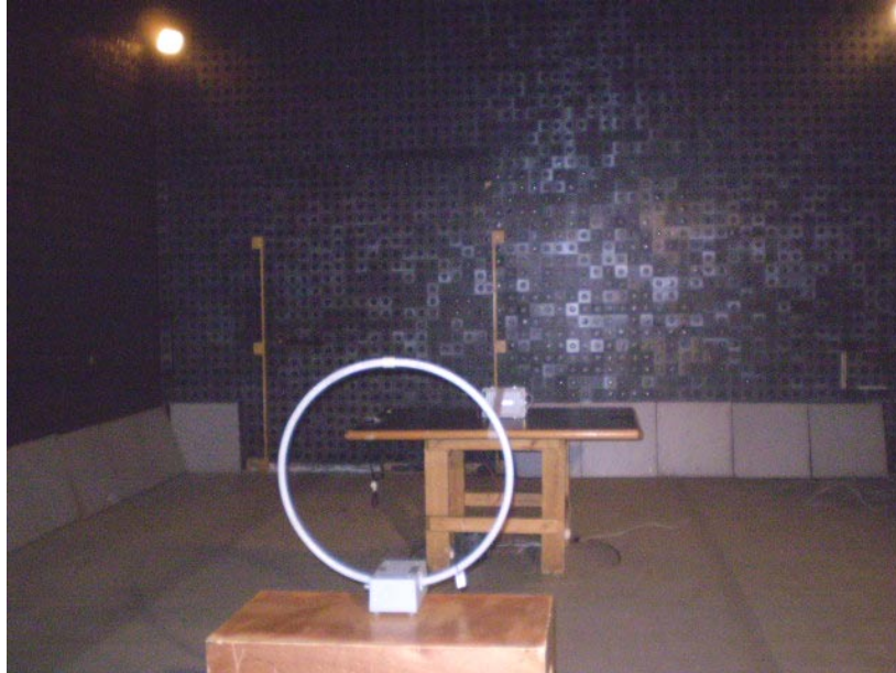
Photograph No.2 Setup for spurious emission field strength measurements in 9 kHz to 30 MHz range in the anechoic chamber
