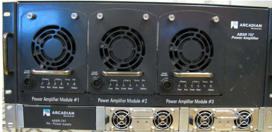
Figure 12: Power Amplifier Front panel (above PA Power supply)
