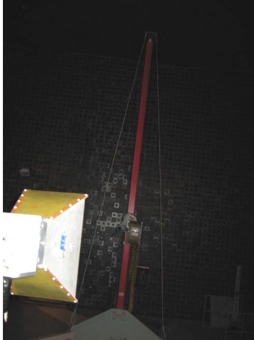
Photograph No.7 Setup for substitution ERP measurements of spurious
