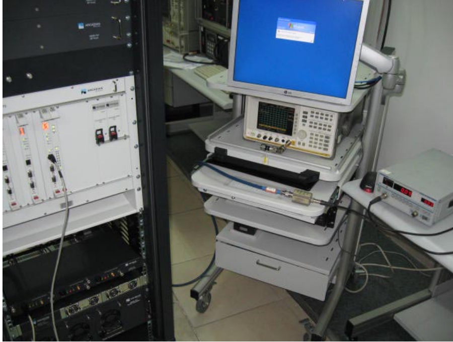
Photograph No.2 Peak output power, occupied bandwidth and spurious emissions at RF antenna connector test setup
