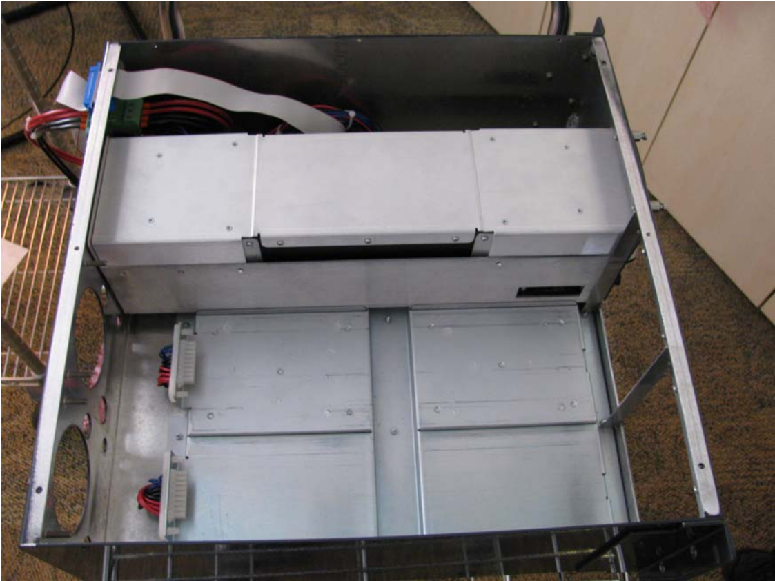
Picture 3: Single RF module in PA box This picture shows the PA box with upper cover removed, and with a single PA module (two PA modules are removed).
