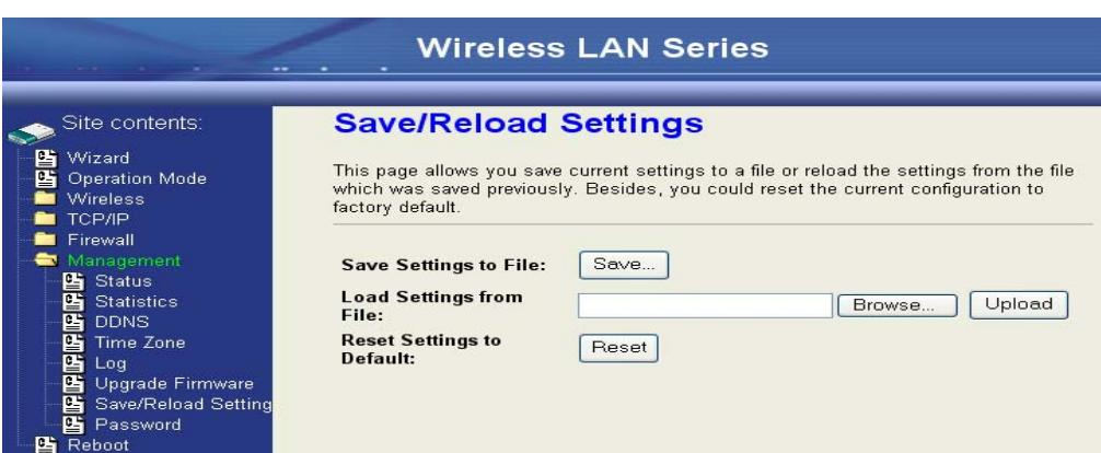
To save & restore configuration data of device, just assign the target filename with full path at your local host, then you can backup configuration data to local host or restore configuration data to the device.
