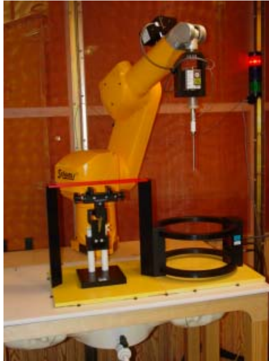
Figure 4.2a T-Coil setup with Helmholtz Coil
