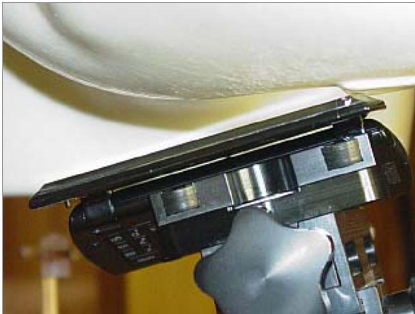
Figure 9E.4 Phone (Open) against the head (Left Tilt position)
