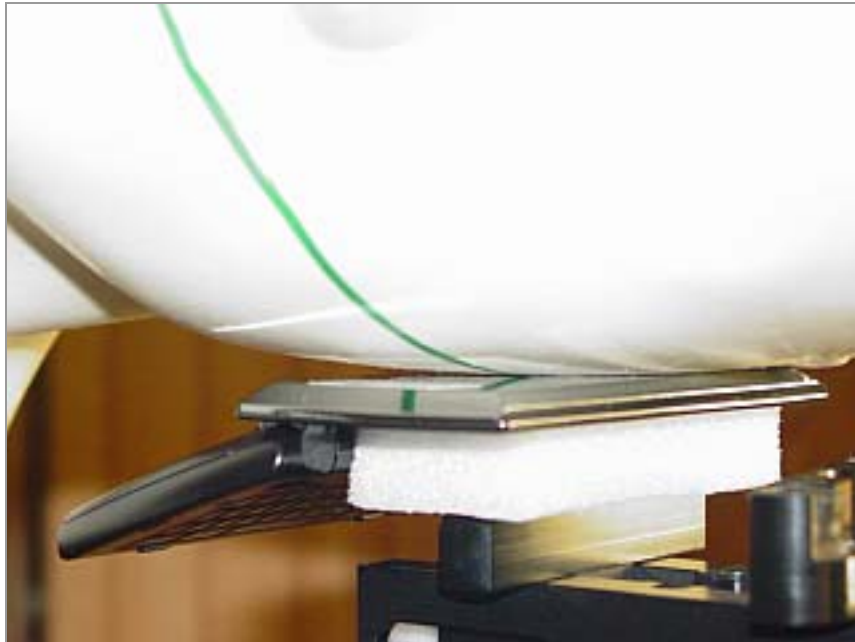
Figure 9E.3 Phone (Open) against the head (Left cheek position)
