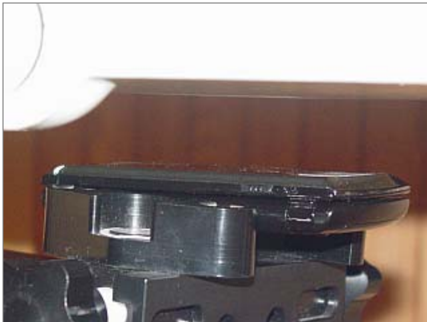
Figure 9E.6 Body SAR setup (Closed, Face Up, 22mm Air Separation)
