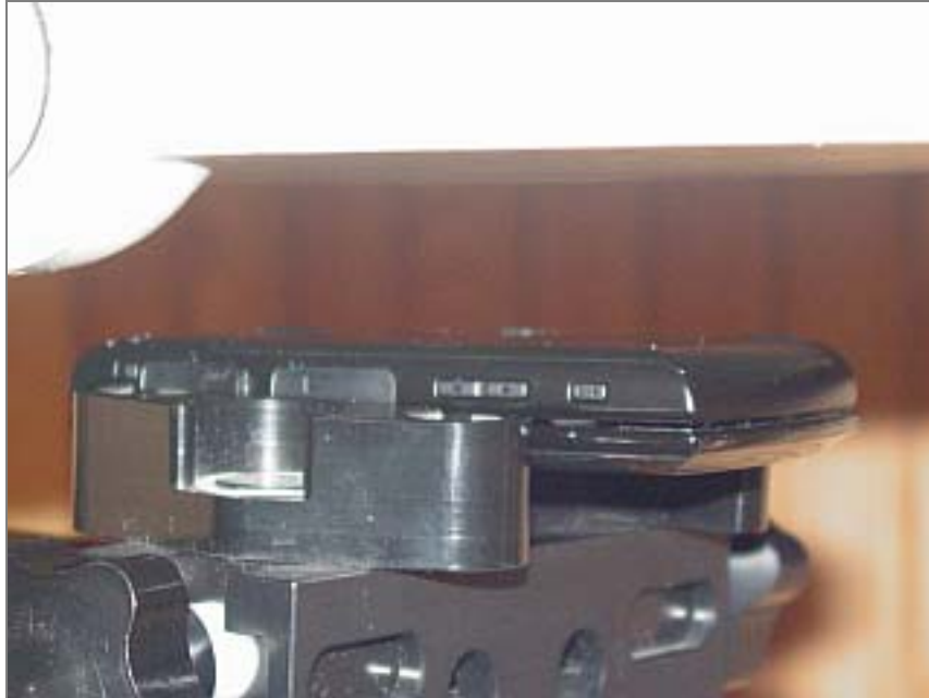
Figure 9E.5 Body SAR setup (Closed, Face Down, 22mm Air Separation)
