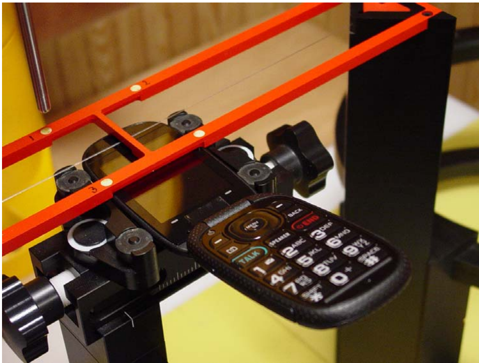
Figure 1a – HAC T-Coil Test Setup
