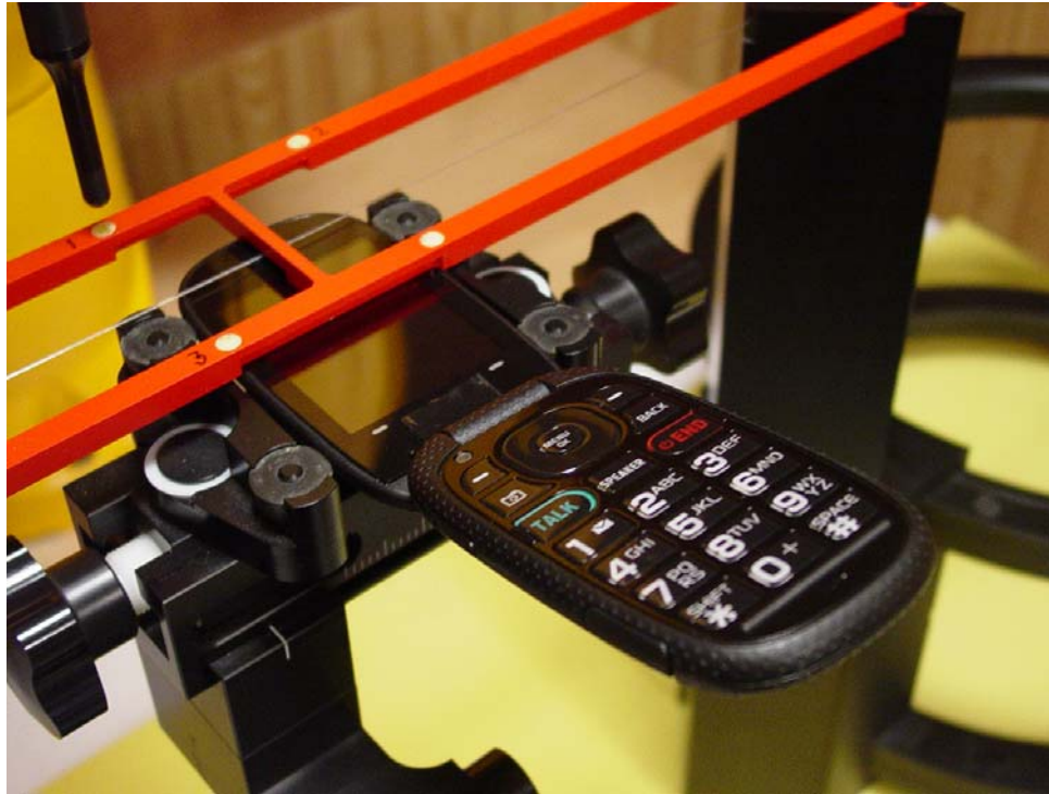
Figure 1a – HAC RF Test Setup
