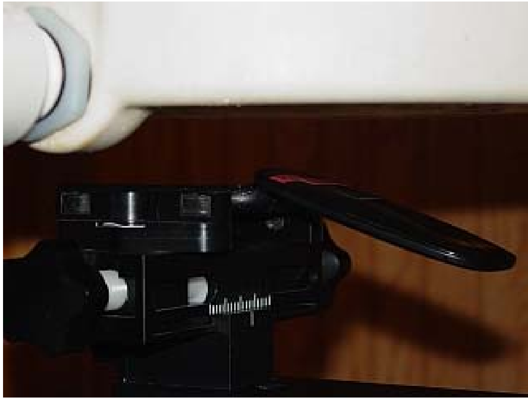
Figure 9E.5 Body SAR setup (Open, Face Down, 22mm Air Separation)
