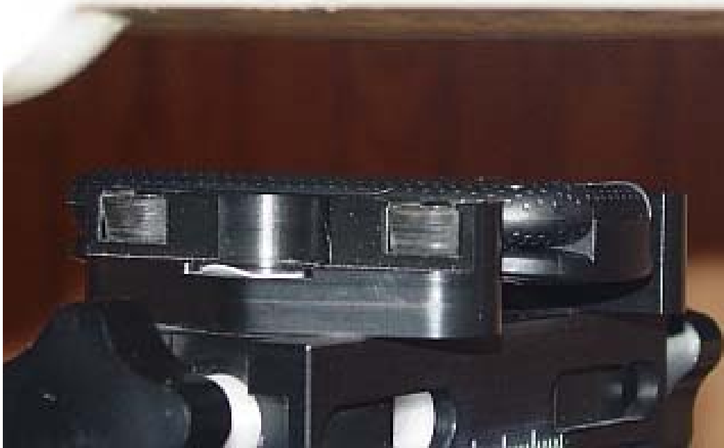
Figure 9E.3 Body SAR setup (Closed, Face Down, 22mm Air Separation)
