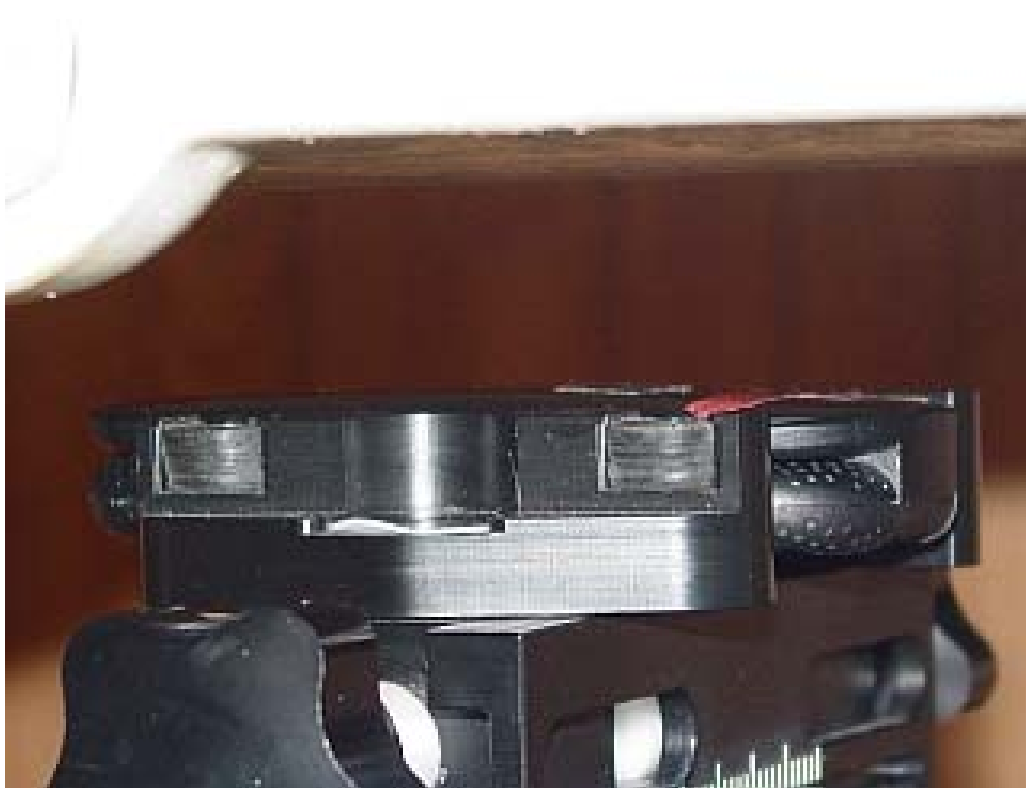
Figure 9E.4 Body SAR setup (Closed, Face Up, 22mm Air Separation)
