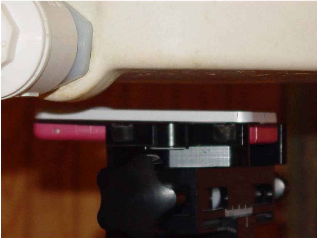
Figure 9E.7 Body SAR setup (Closed, Face Up, 15mm Air Separation)
